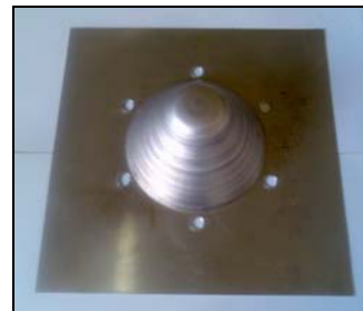
Fig.6. The formed sheet in cone geometry
