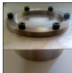
Fig.3. Clamping of annealed Al sheet on the fixture
