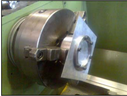
Fig.4. Attaching the fixture on the chuck
