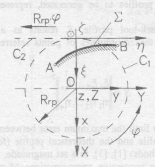
Fig.1. Rack-tool generating scheme.
