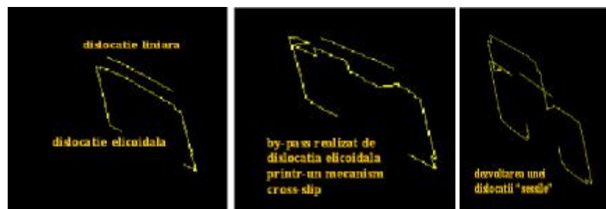
Fig. 5 – Formation of the sessile dislocation by making a by-pass of one dislocation at the intersection of the other dislocation – activation of the secondary slip system
